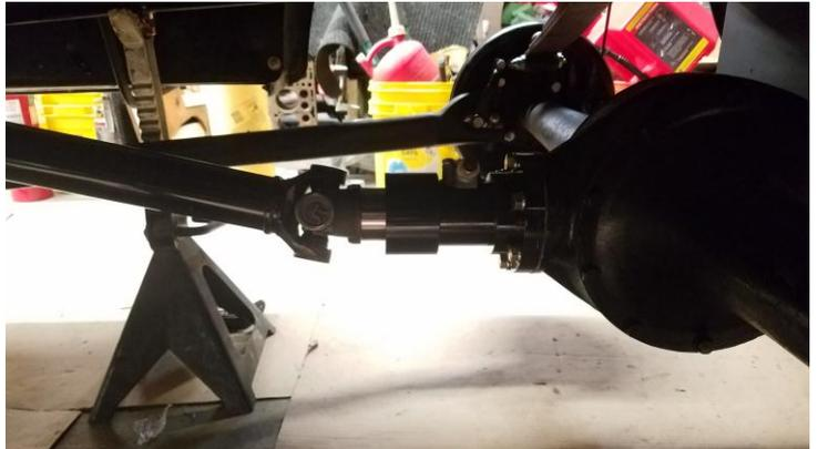
Drive shaft attached to the pinion shaft
