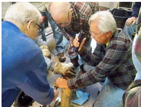
Disassembling differential to diagnose noise. Inspection revealed two broken ring gear teeth.
