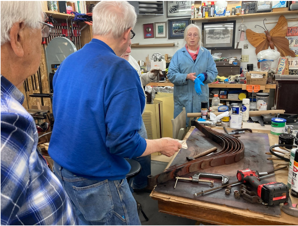
Anne Laviolette's project: George, Ron, Jim, Lee & Anne pulled the motor to resolve rear main leak; we removed & repaired front spring, and reinstalled the engine, then removed & repaired the rear spring. It was a contest at times!
