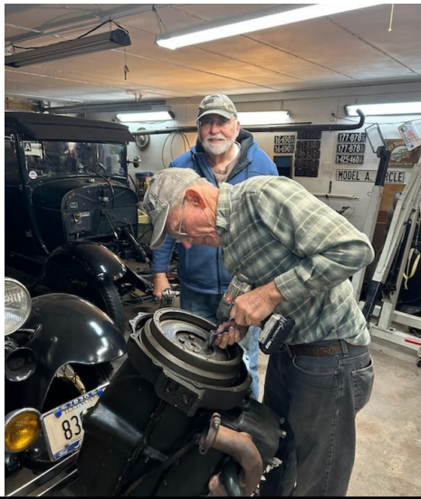
Dave Clark's project: pull the engine out to check the bearings and adjust the valves. Helping Dave were Mike Peters, Lee Laviolette, Bob Nowicki (with the dog), and Mark McClenathan.
