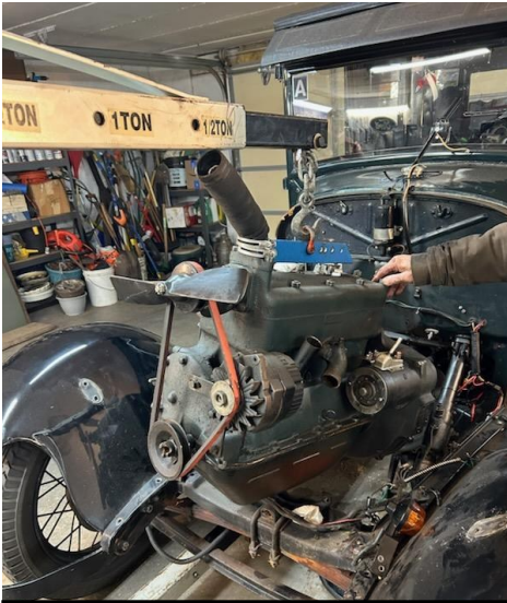
Dave Clark's project: pull the engine out to check the bearings and adjust the valves. Helping Dave were Mike Peters, Lee Laviolette, Bob Nowicki (with the dog), and Mark McClenathan.
